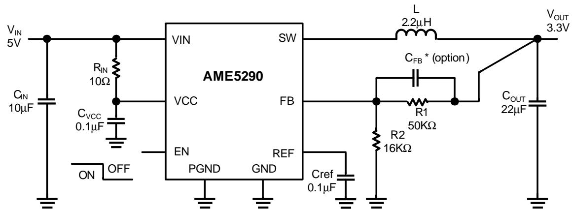
$$V_{OUT} = 0.8V \times \left(1 + \frac{R_1}{R_2}\right)$$
